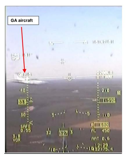
T-38 parameters in this picture are: 353 KIAS, 680 AGL, 1590 MSL, Heading 327, Level Flight.
